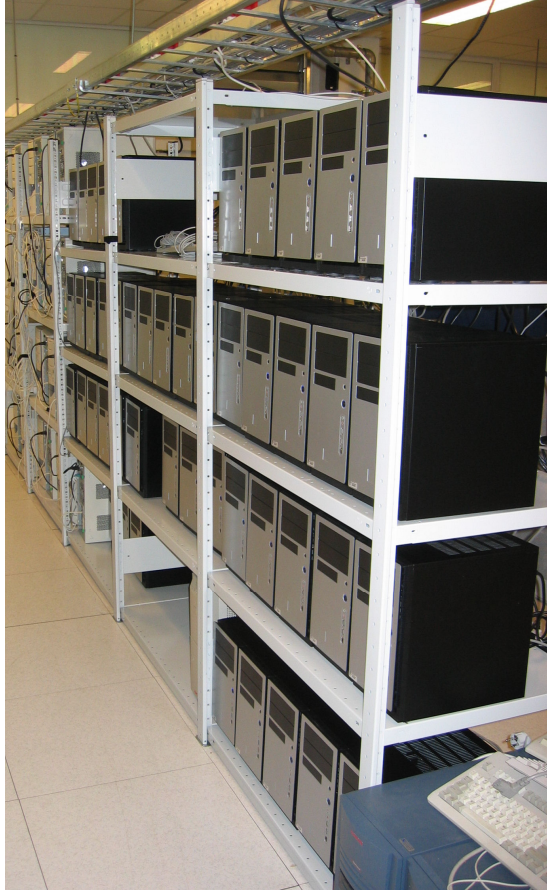
Figure 2.19: Serial computer cluster containing 94 processor cores, specifically selected for 3D Front Tracking calculations.
